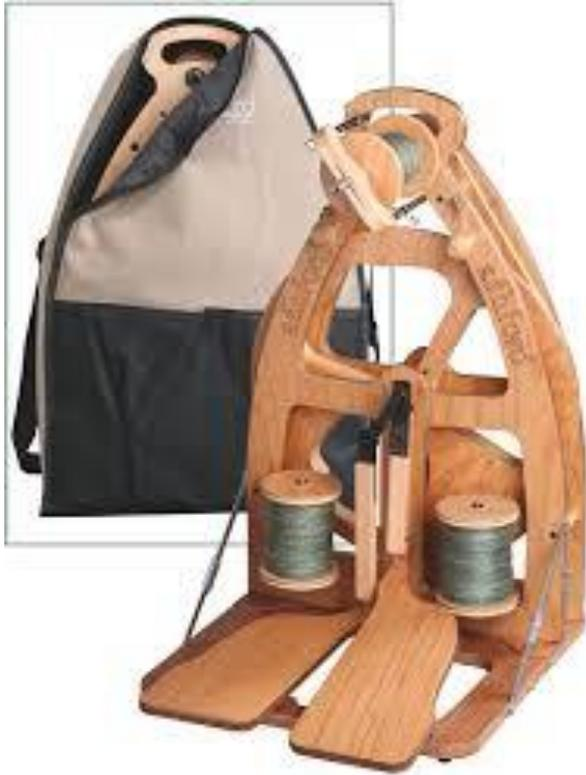
This is a small spinning wheel called a traveller as it folds down into the bag you see in the background, and can be easily transported.
